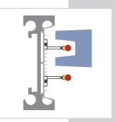
Sample for cable arrangement: Cable in an EMS profile
