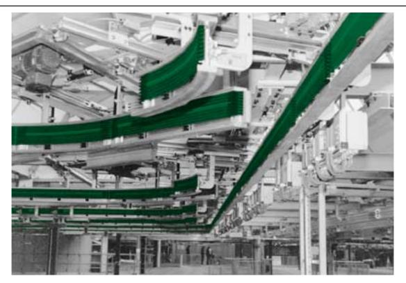
VAHLE U 10 conductors provide power, control and data transmission for automated monorail systems (AMS) in the automative industry.
