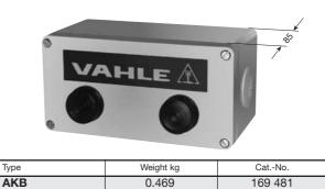
The brush wear indicator will automatically check the brush wear and indicate necessary brush replacement. A continuous axle connected to an enclosed microswitch is equipped with steel feeler pins, arranged between the conductor bars and adjustable to the maximum brush wear level.
